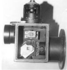
Fig. 9. The interferometer mounted in its cell
