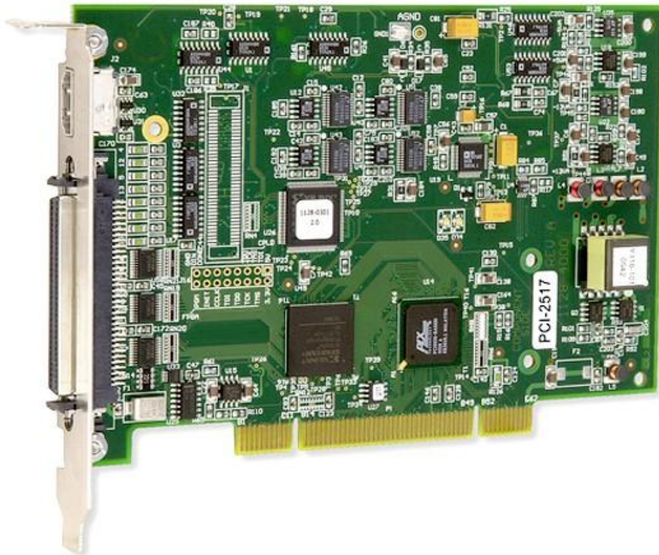
Figure 5. PCI 2517 card which has 16 bit digital I/O, Counters ADC, DAC and Software drivers.
