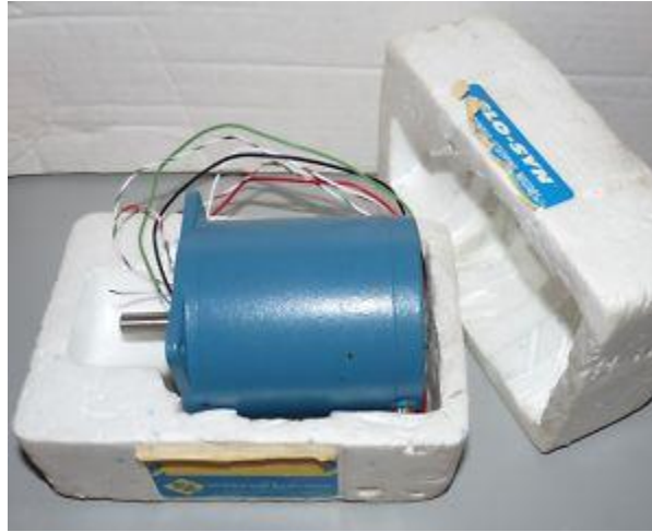
Figure 3. Stepper motor and its specifications.
