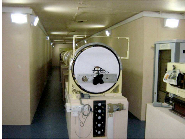
The Littrow-type spectrograph on the Solar Tunnel Telescope
